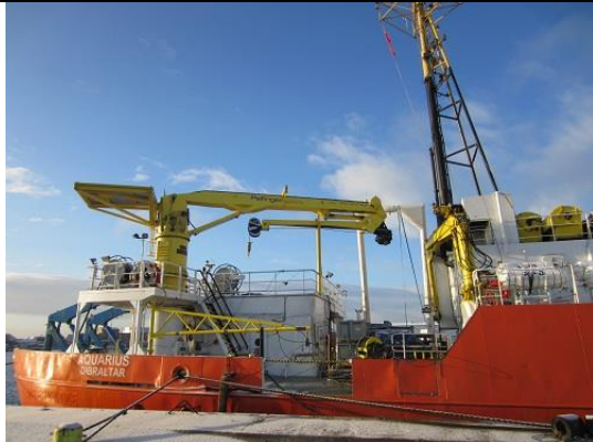
Knuckle JIB-crane with winch platform, out rigger beam for sparker
