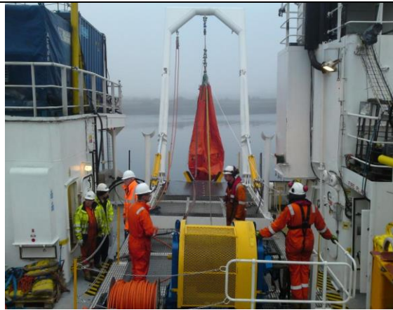
port side A-Frame SWL 8T and Vibrocorer Winch
