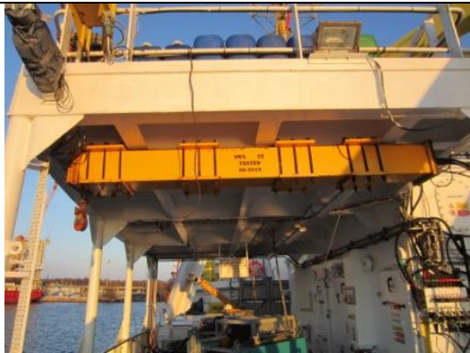
PS horizontal telescoping beam for sidescan operation
